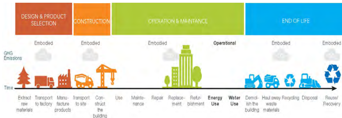
Figure 13 - Various stages and modules for LCA, Source: New Building Institute
