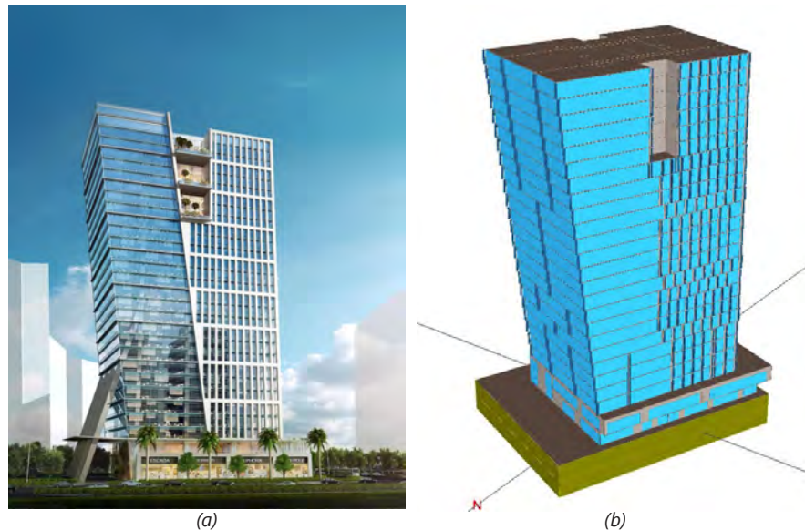
Figure 10 - (a) Actual building, (b) Energy model of the building
